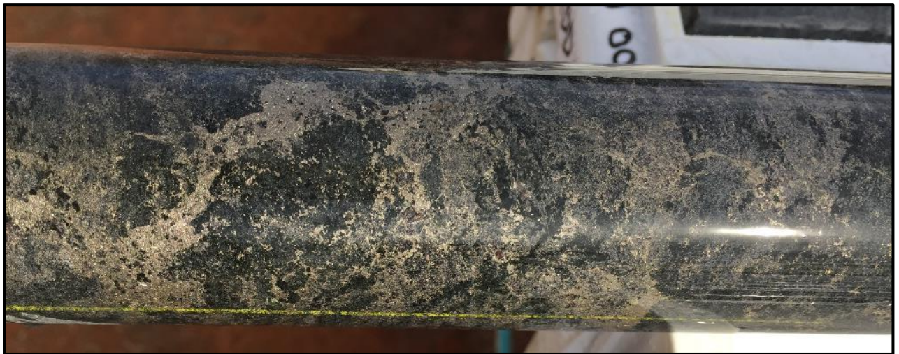
Photo 1: RKDD001-566.8m: Pyrrhotite in mafic granulite (NQ2 core)
