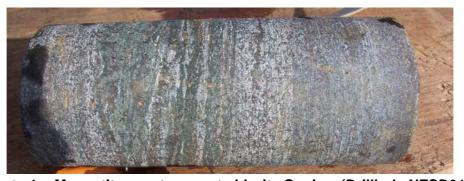
Photo 1: Magnetite-quartz-garnet-chlorite Gneiss (Drillhole NESD011)
