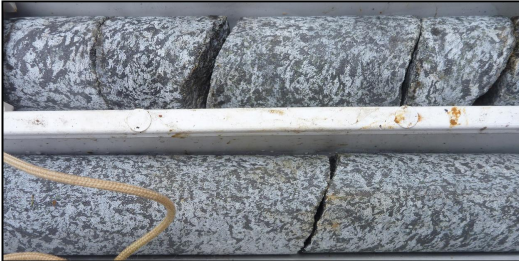
Photo 1 : Magnetite Gneiss Drillcore from Drillhole DH046
