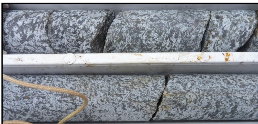
Photo 1: Magnetite Gneiss Drillcore from Drillhole DH046
