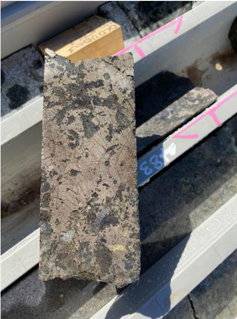
Fig.2. Drill Hole OCDD001 – semi-massive Ni-Cu-Fe sulphides
