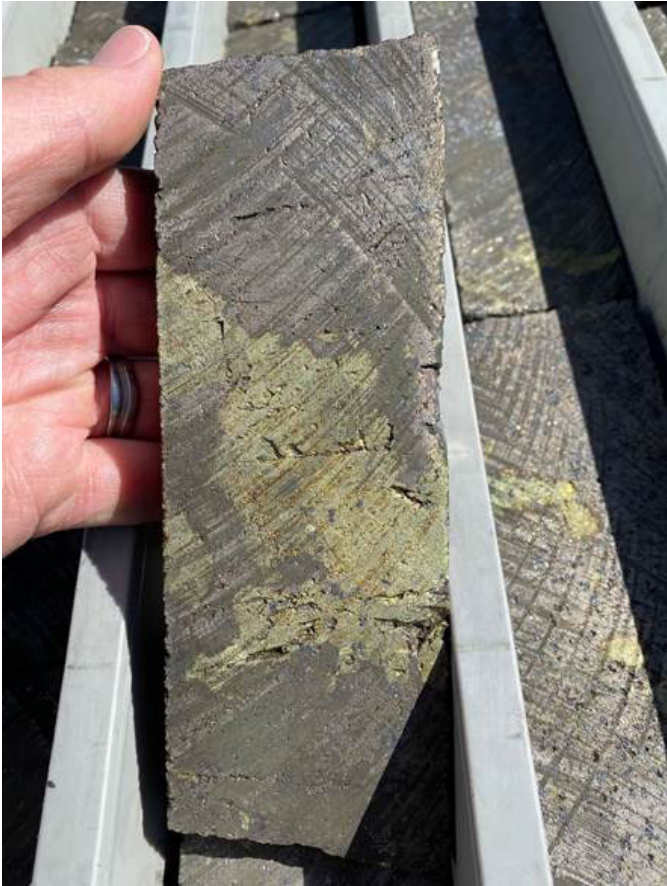
Fig.5. Mawson RKDD034 drill core - 31m @ 2.8% Ni, 2.0% Cu and 0.15% Co from ~201m.
