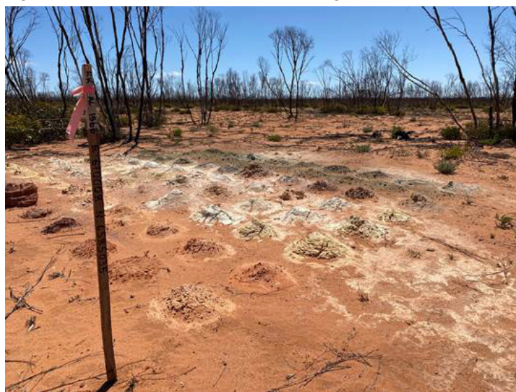
Fig.7. Area W – Aircore site RKAC1566 – 12m @ 0.1% Ni and 0.09% Cu from 58m
